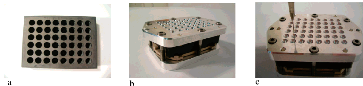
Figure 1. (a) Prototype 48 deep-well microtiter plate ( 82 \times 62.5 \times 18 mm) made of sintered silicon carbide. (b) Sealed microtiter plate setup ( 118 \times 80 \times 46 mm) consisting of the SiC deep-well plate on an alumina base with a PEEK spacer, covered with an alumina top plate with corresponding bore holes for sample withdrawal, and fixed with six stainless steel hex bolts for use in a multimode microwave reactor. For a detailed drawing, see Figure S3 in the Supporting Information. (c) Detailed view of the sealing mechanism. A needle is shown penetrating the \text{\O} 1.2 mm hole in the top aluminum sealing plate, the Viton sealing mat, and the PFA foil to reach inside one well.
